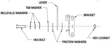
FIGURE 17 THROTTLE TENSION
